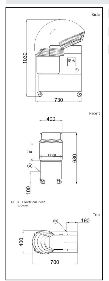
Electric Supply voltage: 380-415V/3 ph/50 Hz **Total Watts:** 1.1 kW Capacity: Maximum kneading (60% hydratation): 17 kg/Cycle Key Information: External dimensions, Width: 400 mm External dimensions, 700 mm Depth: External dimensions, Height: 680 mm 78 kg **Shipping weight: Bowl capacity:** 22 lt
